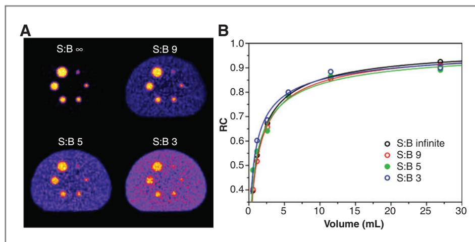
Figure 1.  $^{124}\text{I}$  PET/CT calibration. A, NEMA IEC Body Phantom PET acquisitions with  $^{124}\text{I}$  for spheres to background activity concentration ratios equal to infinite, 9, 5, and 3, conducted to obtain the recovery coefficients (RC; see Materials and Methods) for dosimetric calculations. B, course of the recovery coefficients as a function of sphere volume represented for different S:B concentration ratios.
